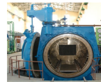
Mark III: Working Space: 2m Dia x 4m Len Max. Temp. 350°C Pressure: 15 bar(g)
