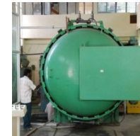
Mark I: Working Space: 2.8 m Dia x 5.2 m Len Max. Temp. 250°C Pressure: 7 bar(g)
