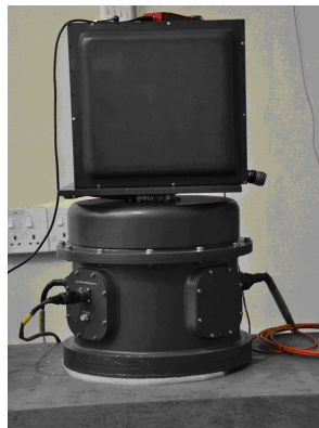
X-band receiving module with 16x16 adaptive array
