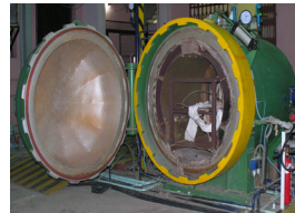
Mark 0: Working Space: 0.9 m Dia x 0.9 m Len Max. Temp. 250°C Pressure: 7 bar(g)
