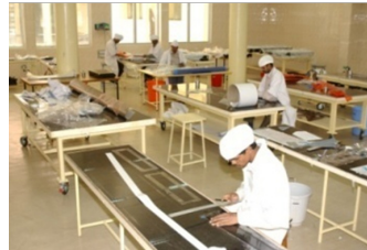
10, 000 class clean room for prepreg layup
