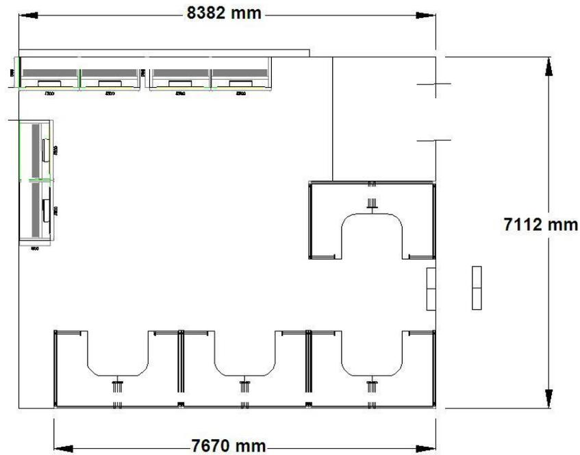
Fig. 1 Layout for Linear and L shaped computer work station tables
