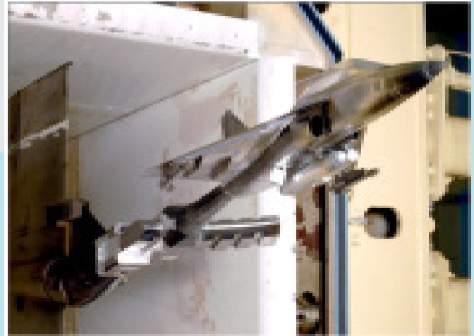
LCA model mounted in the NAL 1.2m wind tunnel
