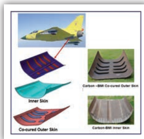
Developmental approach to realize co-cured Engine bay door assembly
