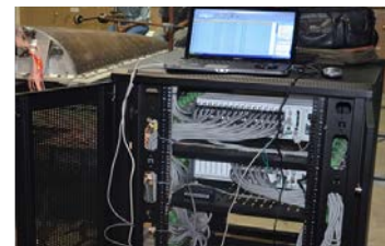
200 channel strain data acquisition system
