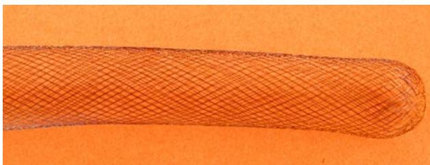
Photograph of Ni-Ti braided mesh using 80 \mu m diameter wire
