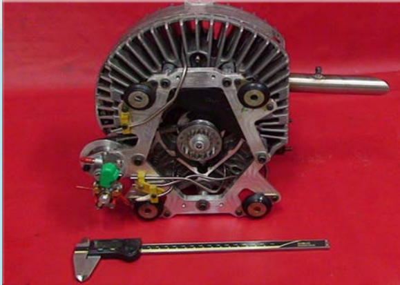
First Prototype 30 hp Wankel Rotary Engine
