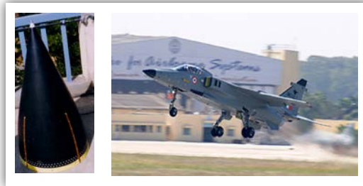
Jaguar nose cone composite radome
