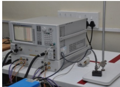
Dielectric Probe: EM characterization of solid
