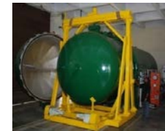
Mark II: Working Space: 1.8m Dia x 4m Len Max. Temp. 200°C Pressure: 7 bar(g)
