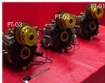
Indigenous 65 hp Wankel Rotary Prototype Engine
