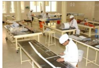
10, 000 class clean room for prepreg layup
