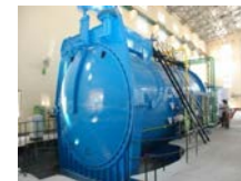
Mark IV: Working Space: 4.4m Dia x 9m Len Max. Temp. 250°C Pressure: 7 bar(g)
