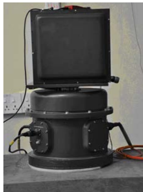
X-band receiving module with 16x16 adaptive array
