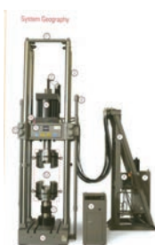
High capacity (100 ton) dynamic axial test system
