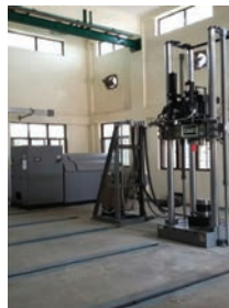
High capacity (100 ton) dynamic axial test system
