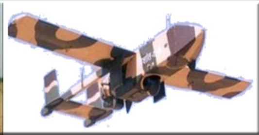
UAV-Nishant maiden successful flight with Wankel engine
