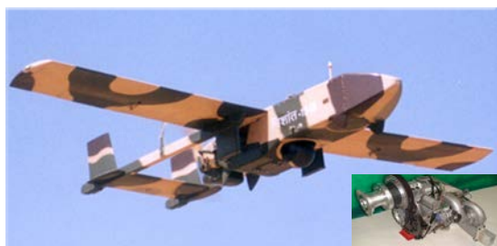
NISHANT UAV maiden successful flight with indigenous 55 hp Wankel Rotary Engine
