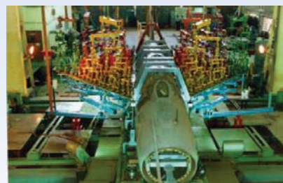
MiG-21 airframe testing
