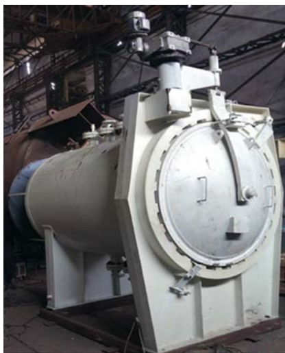
Fig. 21 High temp and high pressure lab scale autoclave for IIT Delhi. Autoclave under fabrication at UCE, Mumbai.
