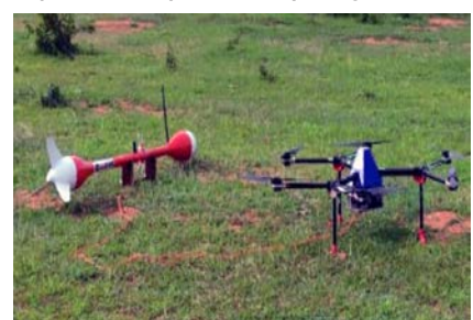
Fig. 15 CSIR-NAL indigenous Hex-copter developed to carry Magnetomer.
