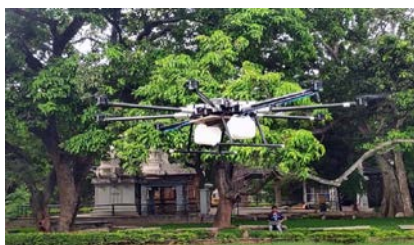
Fig. 14 CSIR-NAL indigenous Octacopter developed to carry Hyperspectral Sensors.
