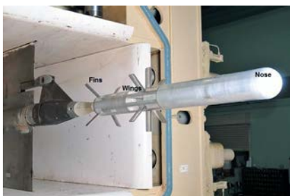
Fig. 16 A photograph of full scale model of typical missile mounted in 1.2 tunnel.
