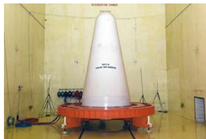
Fig. 18 GSLV-F10, L40 SONC deck acoustic test.
