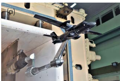
Fig. 8 (a) Saras Mk-2 tractor version wind tunnel model and (b) Surface pressure distribution and wake streamlines for Saras Mk-2 tractor aircraft on power ON conditions.
