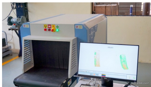
X-ray material discrimination software integrated with baggage scanner
