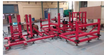
Airframe Assembly JIG
