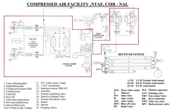
Highlighted portion and the receiver system are proposed for O&M
