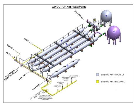
The Compressed Air Facility at CSIR-NAL comprises of a centrifugal compressor plant (2 Compressors - NCAF), along with its associated dryer systems, dryer reactivation systems, cooling water system, water treatment plants and a network of air ducting with air storage receiver system.
