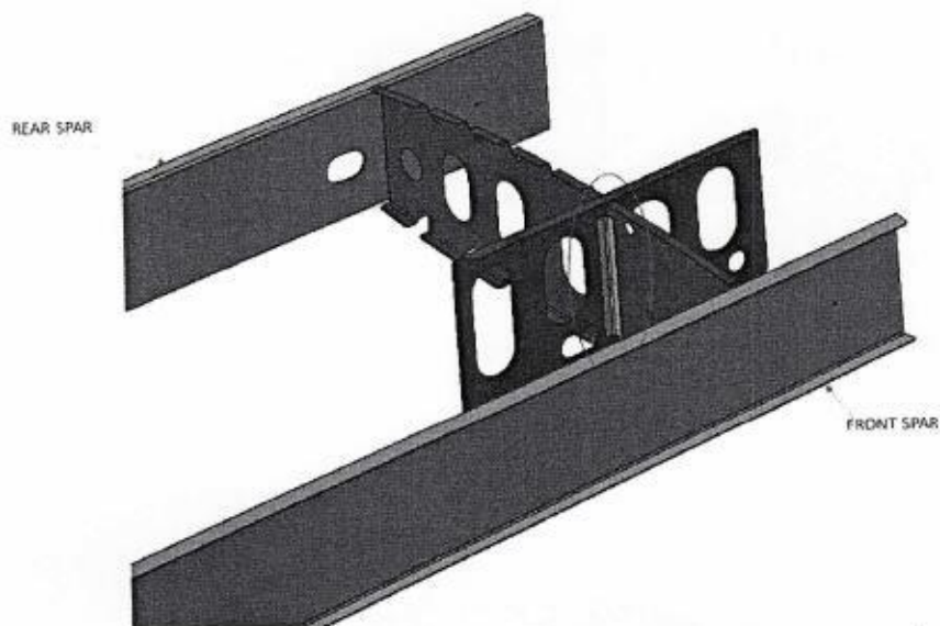
Figure 12. Connecting details of rib # 10 with the SUBSPAR-DRY #9-#11 using L angle
