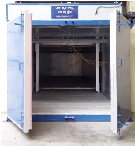
Figure 3: Oven for Post curing
