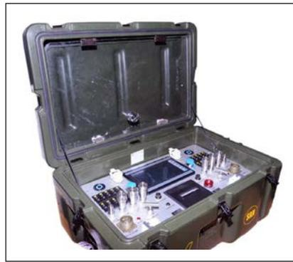
*Fig. 18 Dual zone hot bonder supplied to HAL Bengaluru.*
