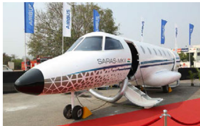
Fig. 4 Physical mock-up of Saras Mk II Fuselage with Interiors, Cockpit, Cabin and ECS system.
