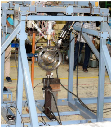
Static test of landing gear of SWIFT UAV
