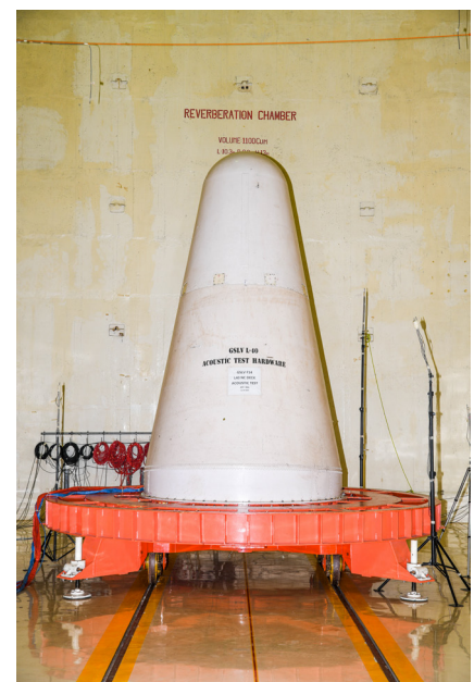
GSLV (F14) -L40 SONC Acoustic Test
