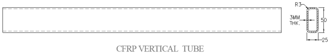
Figure 3. CFRP Vertical Tube (Rectangular Tube) with Dimensions
