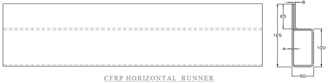
Figure 2. CFRP Horizontal Runner ('P' Tube) with Dimensions
