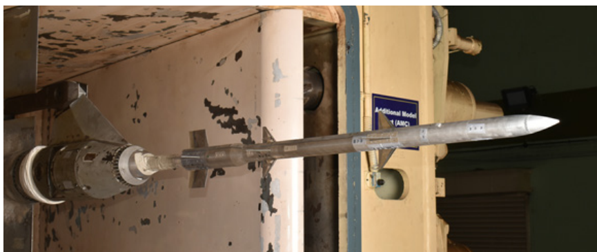
Photograph of a typical missile configuration model mounted in the 1.2 m tunnel.
