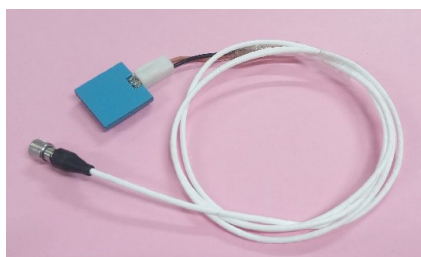
Photograph of developed LTCC-PZT packaged accelerometer prototype
