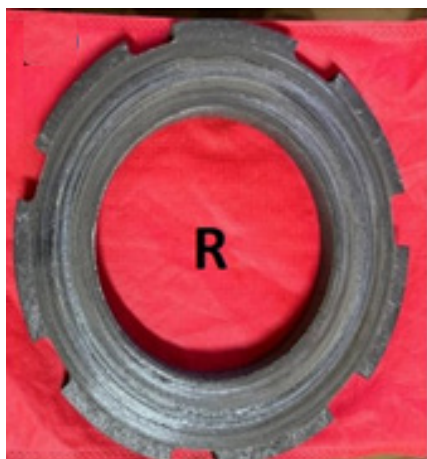
C i /C-SiC composite disks after D-o-D test
