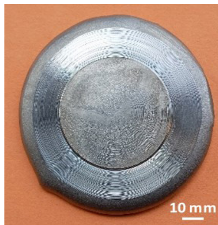
Photograph of melted Ni 50 Ti 30 Hf 20 high-temperature shape memory alloy pancake
