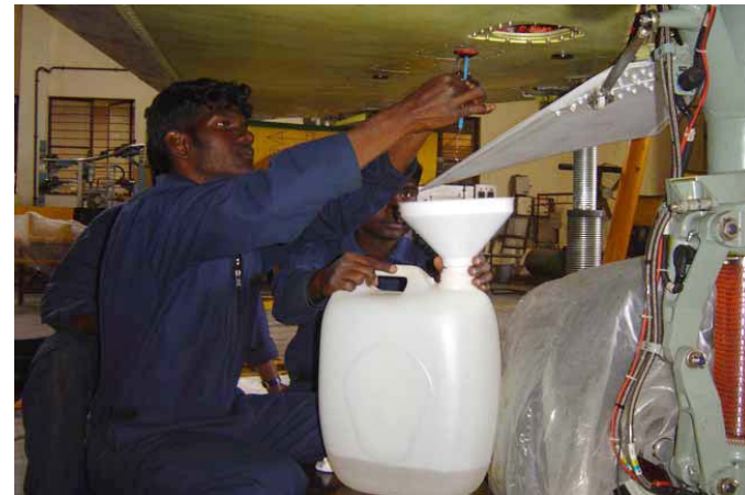
Functional tests of Fuel system
