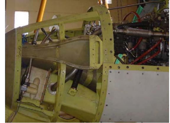
Oil cooler inlet line
