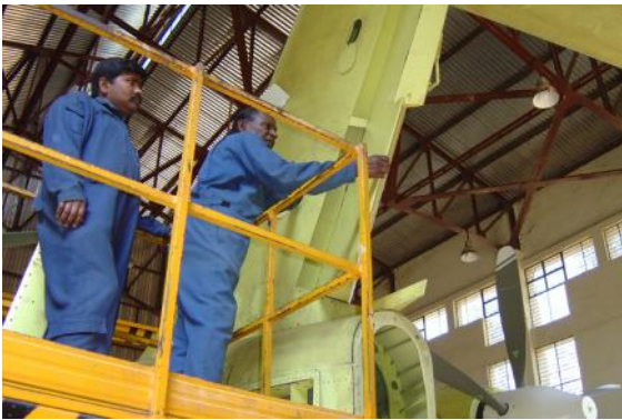
Calibration of trim tabs and FCS movement checks
