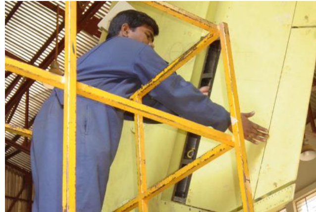
Calibration of trim tabs and FCS movement checks
