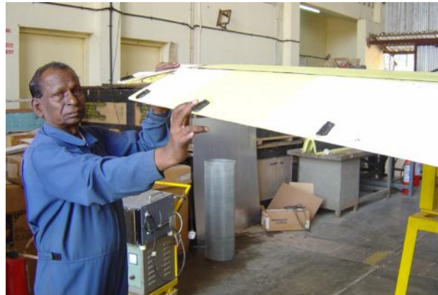
Calibration of trim tabs and FCS movement checks
