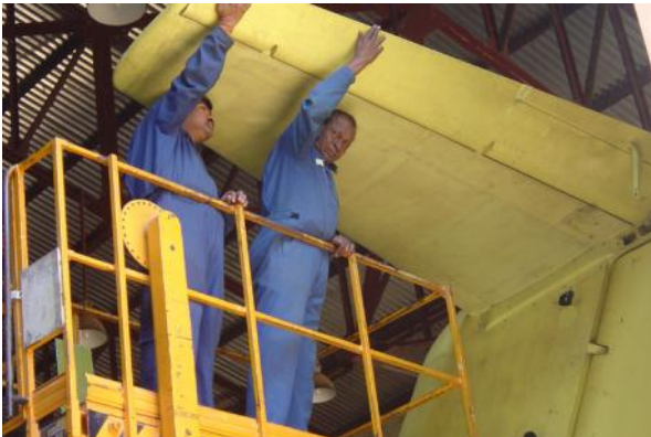
Calibration of trim tabs and FCS movement checks
