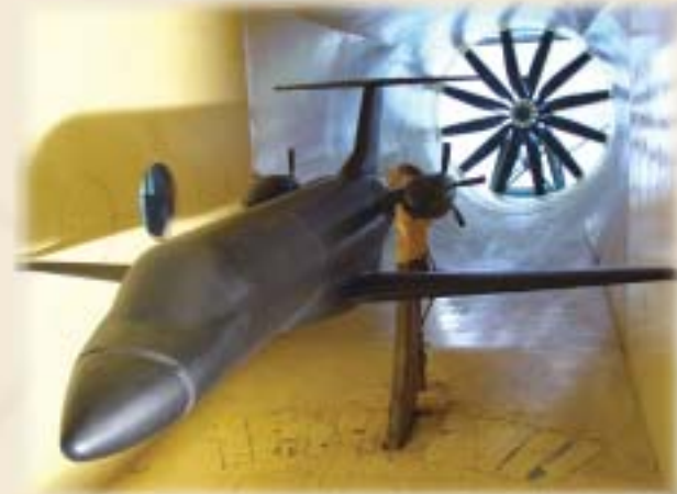
Propeller thrust measurements on an aircraft model
