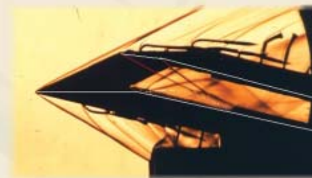
Colour Schlieren photograph of high speed intake flow
