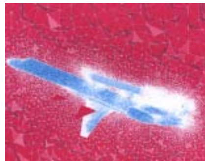
↑ Figure 4 Preliminary design model and the unstructured mesh in the CFD study to measure external flow past an aircraft with dorsal unit.
