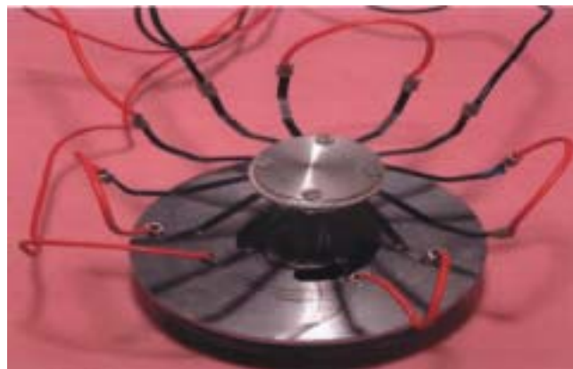
↑ Figure 2 NAL is developing prototypes of smart shape memory alloy (SMA) based repair devices for difficult-to-access areas. The photographs show SMA strips before and after actuation.
