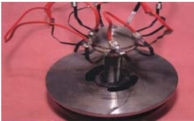
↑ Figure 2 NAL is developing prototypes of smart shape memory alloy (SMA) based repair devices for difficult-to-access areas. The photographs show SMA strips before and after actuation.
