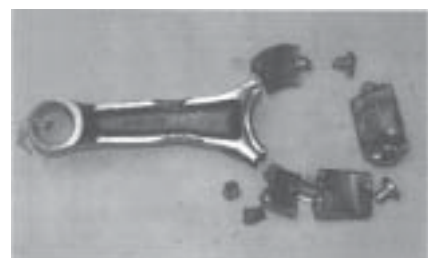
↓ Figure 9: The Materials Science Division investigated the connecting rod failure of the Lycoming engine for HAL.
