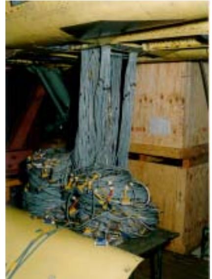
↑ Figure 3: Photograph of the 121 cables, each nearly 50 m long, to be used for the Tejas main airframe structural test specimen.
