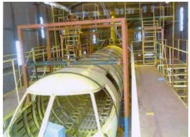
↑ Figure 11: The SARAS fuselage test article being prepared for structural testing.
