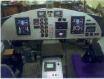
↑ Figure 4: Setup to conduct tests on the navigation systems and primary flight displays of SARAS.
