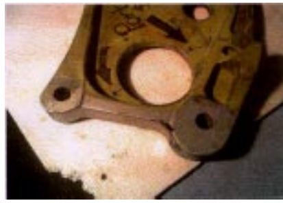
↑ Figure 10: Cracked components of the MiG-21 bis after 16 blocks of loading.
