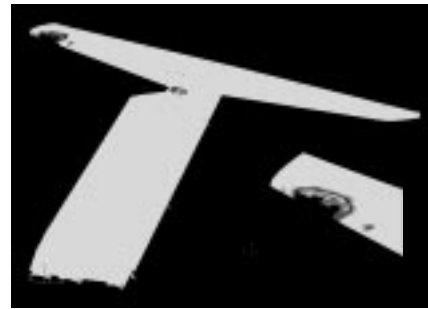
↑ Figure 11: Simulation of the damage to the SARAS horizontal tail after a bird hit.
