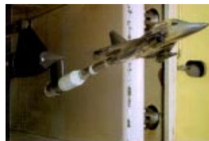
↑ Figure 9: A 1:20 scale LCA naval model mounted in the 1.2m trisonic wind tunnel.
