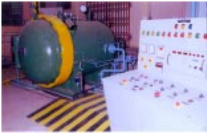
↑ Figure 11 The re-commissioned devine autoclave. Practically the entire autoclave, except the main shell, had to be redesigned and rebuilt.
