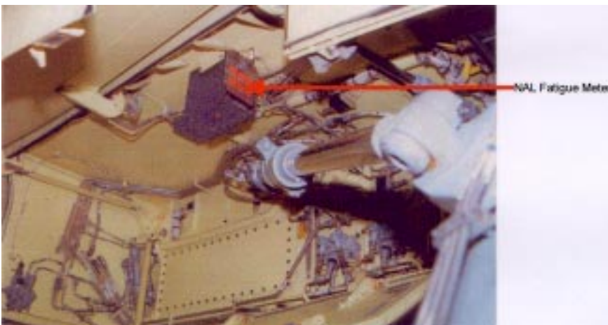
↑ Figure 5 The type-certified electro-mechanical fatigue meter mounted in the undercarriage of the Jaguar aircraft for a flight test.
