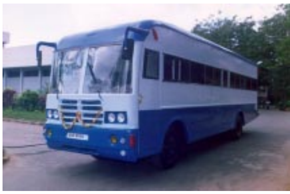
The "low noise" composite van designed by NAL can function as a "travelling clinic" for speech and hearing evaluation.
