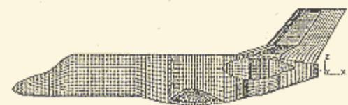
Fig. : SARAS Aircraft Configuration (5811 panels)
