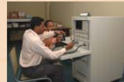
VSWR measurements for antenna and radome
