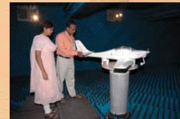
NAL Microwave Anechoic Chamber
