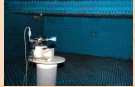
Antenna radiation pattern measurements
