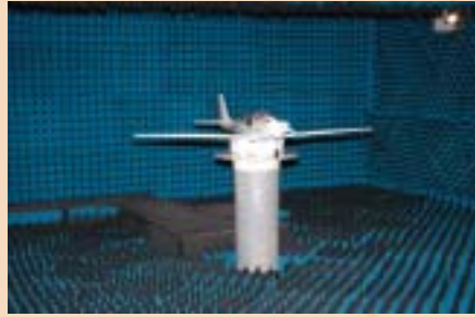
RCS measurements at NAL Microwave Anechoic Chamber (NAL-MAC)
