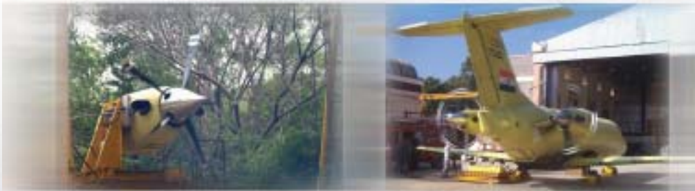
SARAS engine running on test bed and engine test on the aircraft.
