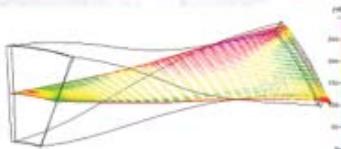
Flow fields in a centrifugal compressor blade passage.
