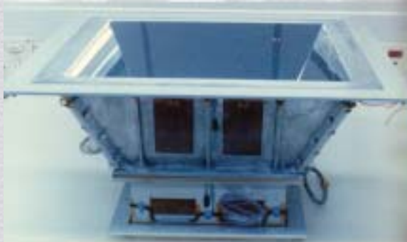
Passive radiative cooler with the four polished mirrors.
