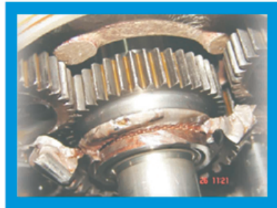
Failed gearbox assembly of an aircraft engine
