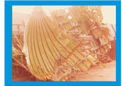
Wreckage of the Kanishka floor structure retrieved from the Atlantic Ocean
