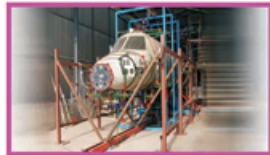
Test set-up of the SARAS fuselage
