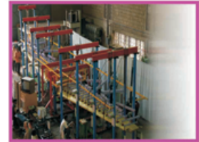
Static test of the SARAS wing
