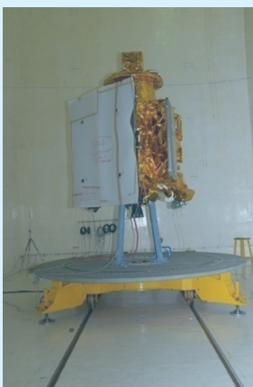
Acoustic test for Chandrayan at CSIR- NAL.
