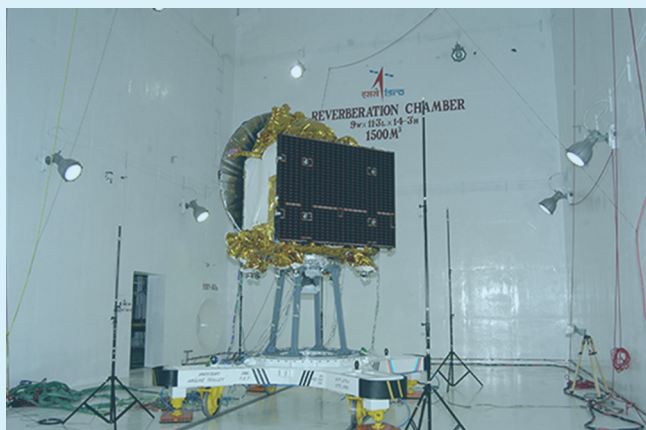
Acoustic test carried out at ISITE(ISRO)-ATF by CSIR-NAL scientists
