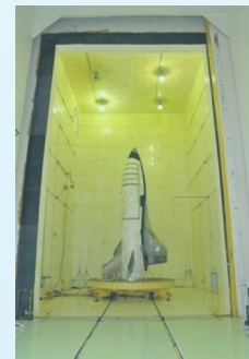
RLV-TD positioned in the reverberation chamber for acoustic test
