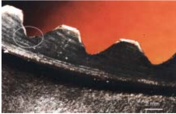
Figure 8. Fatigue cracks at the spline roots.
