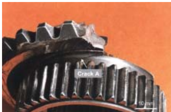
Figure 6. Progressive propagation of crack A in the hub of spur gear.
