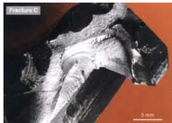
Figure 5. Close-up view of fracture C (refer Fig.2); note the beach marks' orientation.
