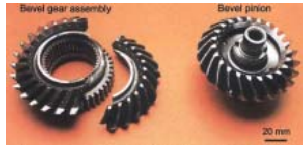
Figure 1. Damaged components of the engine gearbox.
