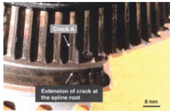
Figure 7. Crack A and extension of a crack at spline root.
