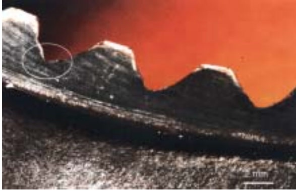
Figure 8. Fatigue cracks at the spline roots.
