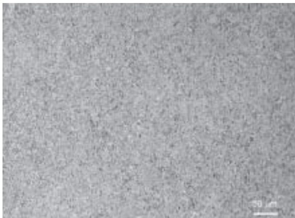
Figure 20. Optical microstructure of the bevel gear teeth case, showing typical carburised structure; etched in 2% Nital solution.
