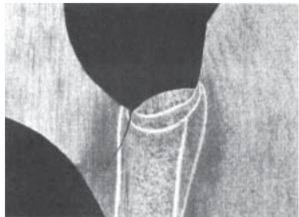
Figure 21. Photograph showing crack at the weld; etched in 2% Nital solution.
