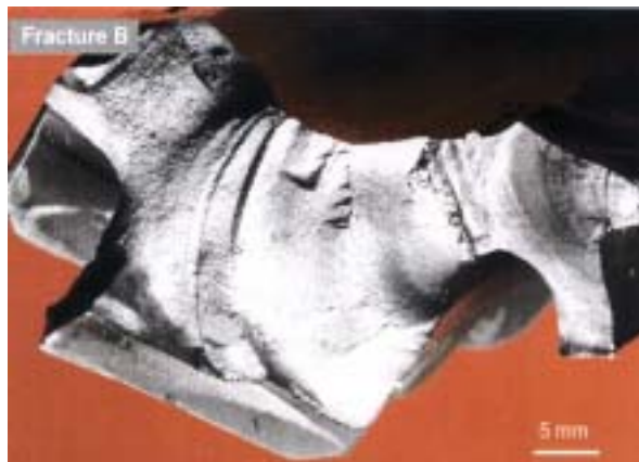
Figure 4. Close-up view of fracture B (refer Fig.2); note the beach marks' orientation.
