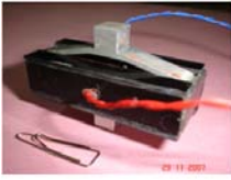
Actuator, Piezo ceramics sensor/ actuator for vibration control
