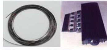
Shape memory alloy as control surface actuator / skin morphing
