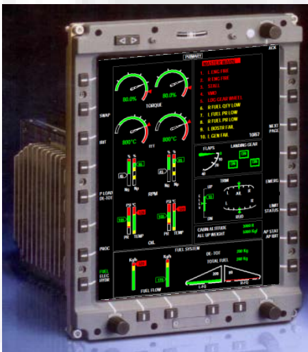
The display system is certified to DO 178B Level A, DO 160F and DO 254 Level A.
