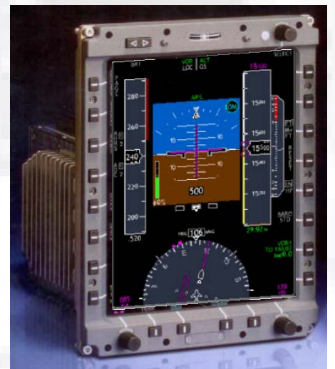
The display system is certified to DO 178B Level A, DO 160F and DO 254 Level A.
