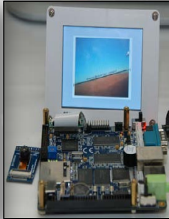
Onboard Vision system for GPS navigation on a Single Board Computer
