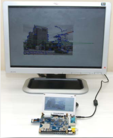
Onboard Vision system for GPS navigation on a Single Board Computer
